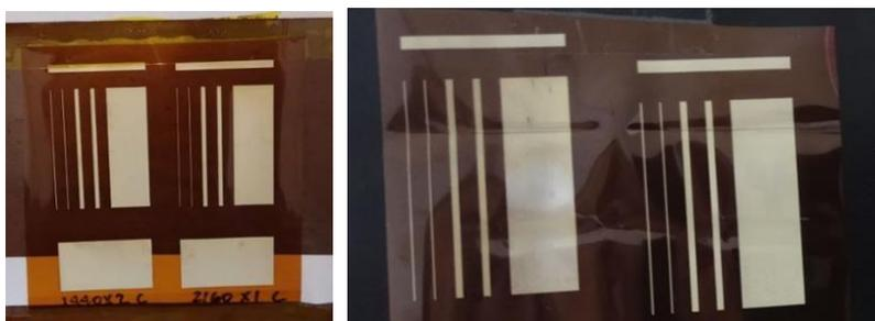
Figure 8: Silver ink "I50TM-119" on Kapton foil. (left) After printing and drying and (right) after sintering and 180 ° bending test.
