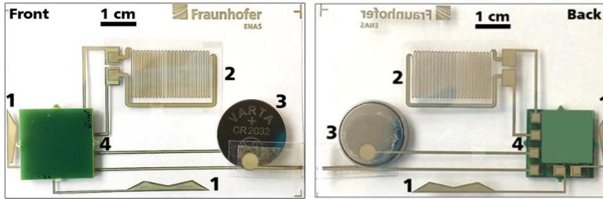
Figure 58: Wireless low power sensor board with printed antenna: (1) 2.45 GHz antenna, (2) temperature sensor, (3) battery and (4) Bluetooth chip.
