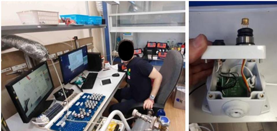
Figure 37: MOX gas sensor demonstrator (RIIT).
