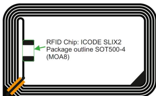
Figure 6: Nearfield RFID NFC communication tag for digital sensor labeling.
