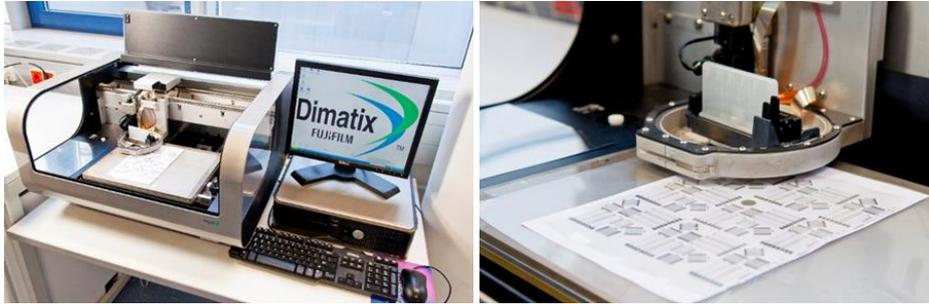
Figure 20: Fujifilm Dimatix inkjet printer DMP-2831 with 10 pl print head.
