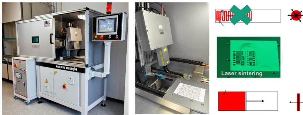
Figure 26: High-power diode laser sintering (HPDL) of printed films.
